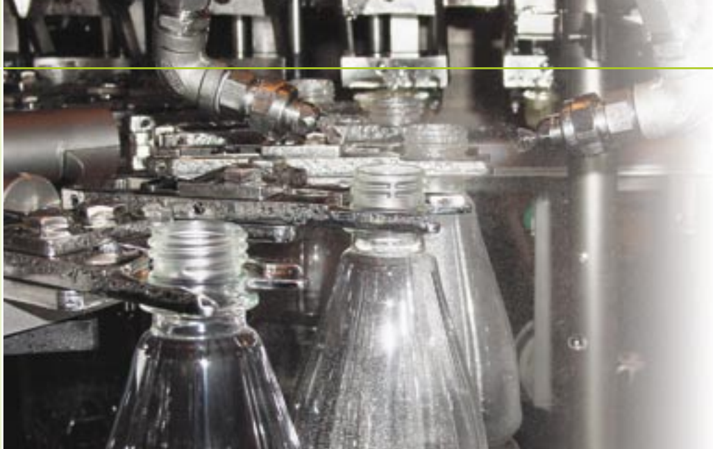
Desinfection of the bottle neck finish with ClO 2 treated water
