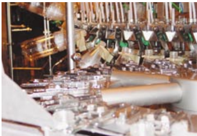
PET mineral water bottles in the rinser
