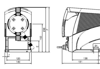
P\_DE\_0046\_1\_SW3 Dimensional drawing of delta® without bleed valve, Material version NP - dimensions in mm
