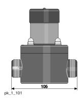
Adjustable back pressure valve for installation in the metering line to generate a constant back pressure and/or for precise metering with a free outlet and with priming pressure on the suction side.
