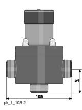
Adjustable relief valve for installation in the metering line to protect against overpressure. With additional connector for the relief line at the base of the valve body, no T-piece is required for installation.
