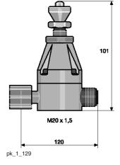
Adjustable back pressure valve for fitting directly onto the dosing head to generate a constant back pressure. For accurate metering with a free outlet and with priming pressure on the suction side.
