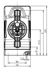
P\_G\_0057\_SW3 Dimensional drawing of gamma/ X, Material design PVT – dimensions in mm
