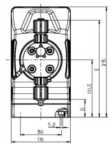
P\_G\_0056\_SW3 Dimensional drawing of gamma/ X, Material design NPT – dimensions in mm
