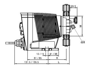
P\_BE\_0071\_SW3 Dimensional drawing of Beta®, Material version PV - dimensions in mm
