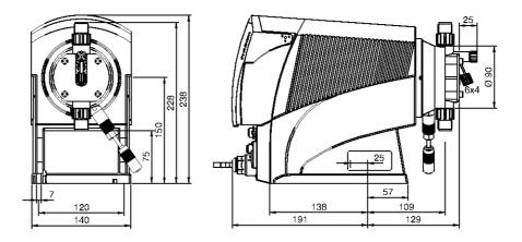
P\_DE\_0042\_SW\_2\_SW3 Dimensional drawing of delta® type 1612-0730, Material version PV - dimensions in mm
